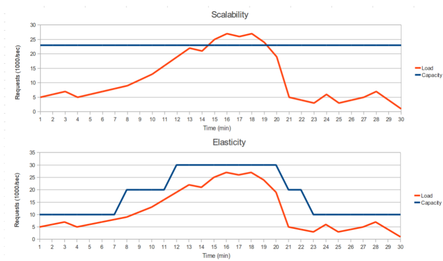
Figure 10 : Comparison of Scalability and Elasticity. Adopted from Figure I.1 of [19]
