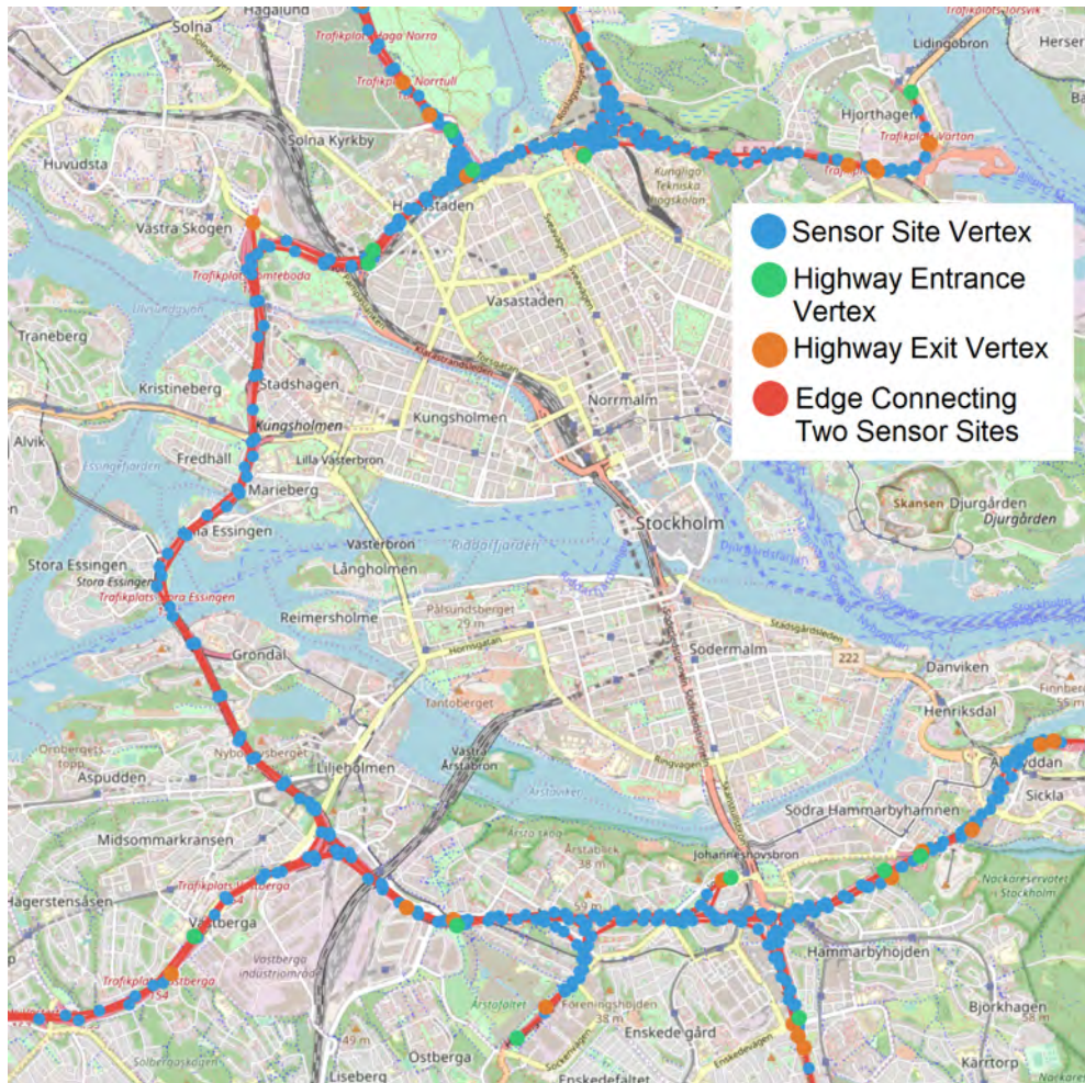
Figure 6.4: Trafikverket’s traffic sensor site graph overlaid of Stockholm center on top of a map
