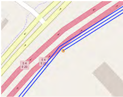
(a) Dummy vertex at the start of a new lane. E4N just north of Södertälje.
