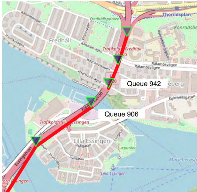
Figure 5.17: Adjacent queues. Two different queues are visible in the image, the one towards the bottom of image with ID 906 and the one in the top half with ID 942. The queues are separated by a non-congested road segment. Triangles represent the traffic sensors and the red lines represent congested links. Results from congested components, for test congestion pattern 3, E4N component 7, 2016-11-1 11:30, with congestion class threshold 5.
